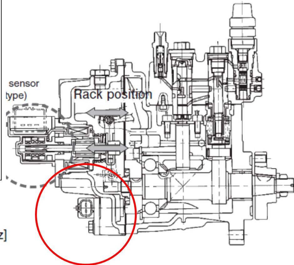
$$Nrpm [\text{min}^{-1}] = (fp \times 2/12) \times 60 = 10 \times fp [\text{Hz}]$$
